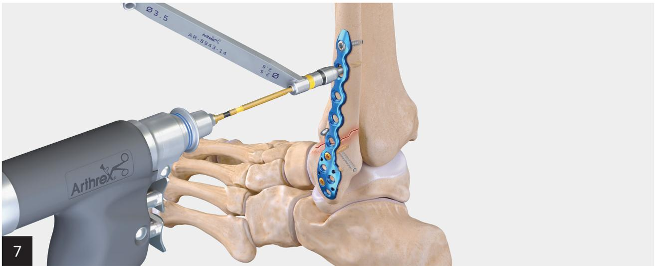
Remove the BB-Tak and replace with a 3.5 mm cortical screw. Drill with the **2.5 mm drill bit** through the **3.5/2.5 mm drill guide**. Measure with the **2.7/3.5/4.0 mm depth device**. Use a **T15 driver** for insertion. This technique can also be used for any proximal 3.5 mm cortical screws. Add additional screws proximally and distally as needed.
