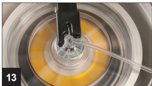
13 The Angel system can process 40 - 180 mL of whole blood, bone marrow aspirate, or a mixture of both in a single cycle. The approximate spin time for a 40 mL sample is 15 minutes. The spin time for a 180 mL sample is 26 minutes.
