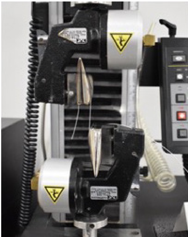
Figure 1. Straight-pull test setup
